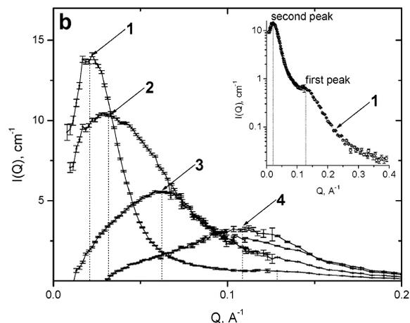
**Figure 12.** SANS profiles for charged C12-20% (a) and C8-20% (b) HM PAA gels with a fixed polymer concentration (30 wt %) and different contents of charged carboxylic groups: (1) 1 mol %; (2) 2 mol %; (3) 4 mol %; (4) 6 mol %; (5) 20 mol %. In the insets, some of the curves are presented in logarithmic scale.
