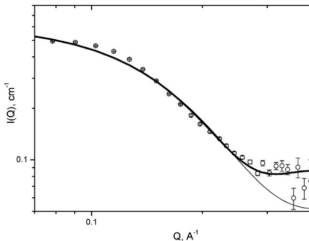
**Figure 5.** The scattering curve of the uncharged C8-5% gel (swollen by D<sub>2</sub>O) (circles) and the fits of experimental data by the form factors of an ellipsoid with the semiaxes of  $10 \pm 2 \text{ \AA}$  and  $19 \pm 2 \text{ \AA}$  (normal line) and a sphere with the radius of  $14 \pm 2 \text{ \AA}$  (bold line). The polymer concentration is 10 wt %.
