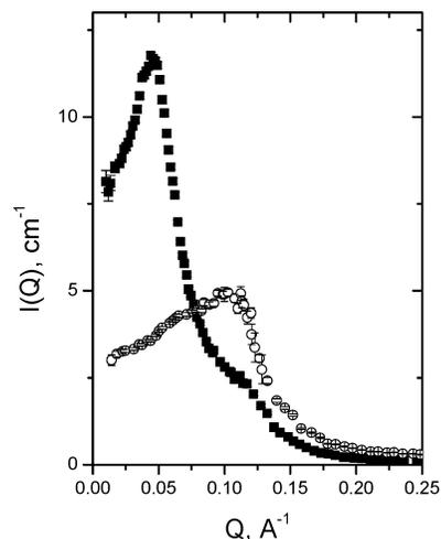
**Figure 16.** SANS profiles for charged C12-20% gels with fixed polymer concentration (30 wt %) and content of charged groups (4 mol %) in the absence of salt (circles) and in the presence of 0.077 mol/L NaCl (squares).
