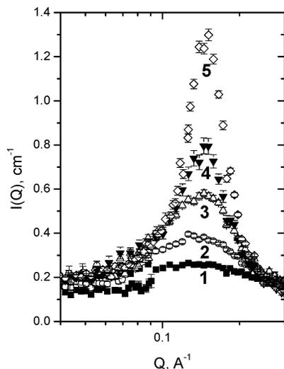
**Figure 10.** SANS profiles for HM PAA C8 gels containing 20 mol % of charged units with a fixed polymer concentration (60 wt %) and different contents of the hydrophobic units: (1) 2.5 mol %; (2) 5 mol %; (3) 10 mol %; (4) 15 mol %; (5) 20 mol %.
