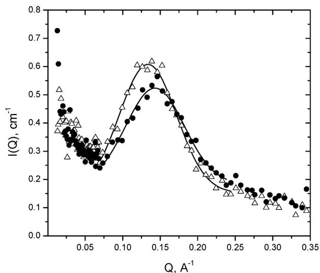
**Figure 8.** SANS profiles for uncharged HM PAA gels C8-20% (swollen by D<sub>2</sub>O at pD = 3) before (dark circles) and after (triangles) the absorption of benzene (the sample with absorbed benzene contains 1 mol of benzene per 1.15 mol of hydrophobic side chains). The polymer concentration is 77 wt % in both cases. The solid lines were obtained by approximation of the experimental data by a Gaussian function.
