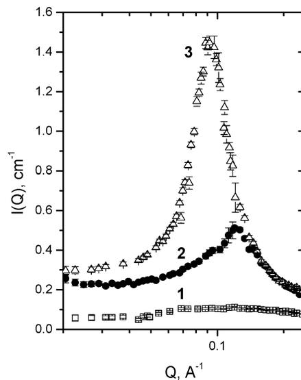
**Figure 4.** SANS profiles for uncharged HM PAA gels (swollen by D<sub>2</sub>O at pD = 3) with *n*-alkyl chains of different lengths: *n*-octyl (1), *n*-dodecyl (2), and *n*-octadecyl (3). In all samples, the polymer concentration is 60 wt %, and the content of hydrophobic units is 2.5 mol %.
