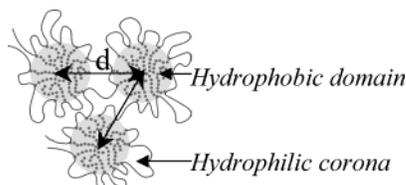
**Figure 7.** Schematic representation of the HM gel structure.
