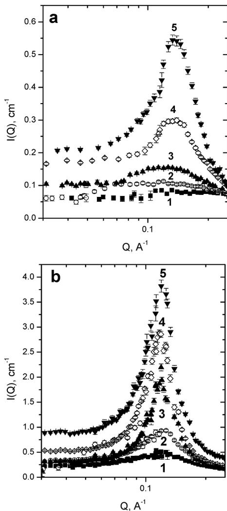
**Figure 3.** SANS profiles for uncharged HM PAA gels (swollen by D<sub>2</sub>O at pD = 3) with fixed polymer concentration (60 wt %) and different contents of *n*-octylacrylate (a) repeat units ((1) 0 mol %; (2) 2.5 mol %; (3) 5 mol %; (4) 10 mol %; (5) 20 mol %) and *n*-dodecylacrylate (b) repeat units ((1) 2.5 mol %; (2) 5 mol %; (3) 10 mol %; (4) 15 mol %; (5) 20 mol %).
