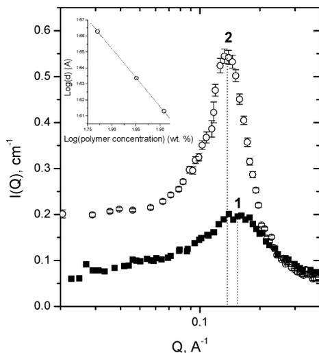
**Figure 6.** SANS profiles for uncharged C8-20% gels with different polymer concentrations: (1) 80 wt %; (2) 60 wt %. In the inset: the dependence of characteristic distances  $d$  on the polymer concentration. The slope of the straight line is equal to  $-0.35$ .
