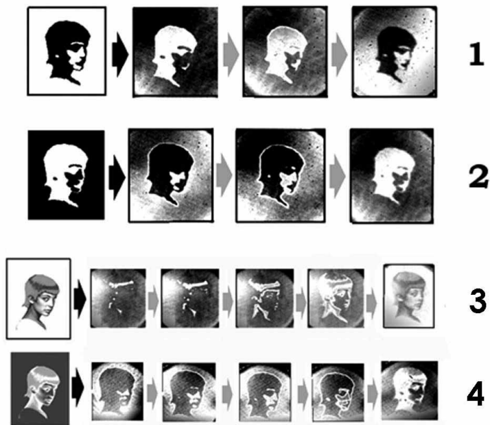
FIGURE 3 Processing black and white (positive – 1, and negative – 2) and half-tone (positive – 3, and negative – 4) images by a chemical reaction-diffusion medium.
